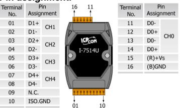
Pin 11/13 and Pin 12/14 Easy-to-use wiring for RS-485 in a daisy chain configuration.
